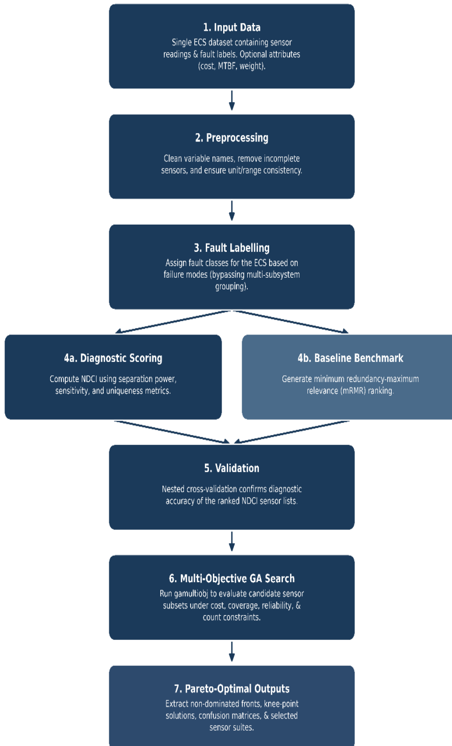
Figure 3-8 NDCI MOSOF pipeline in ECS case
